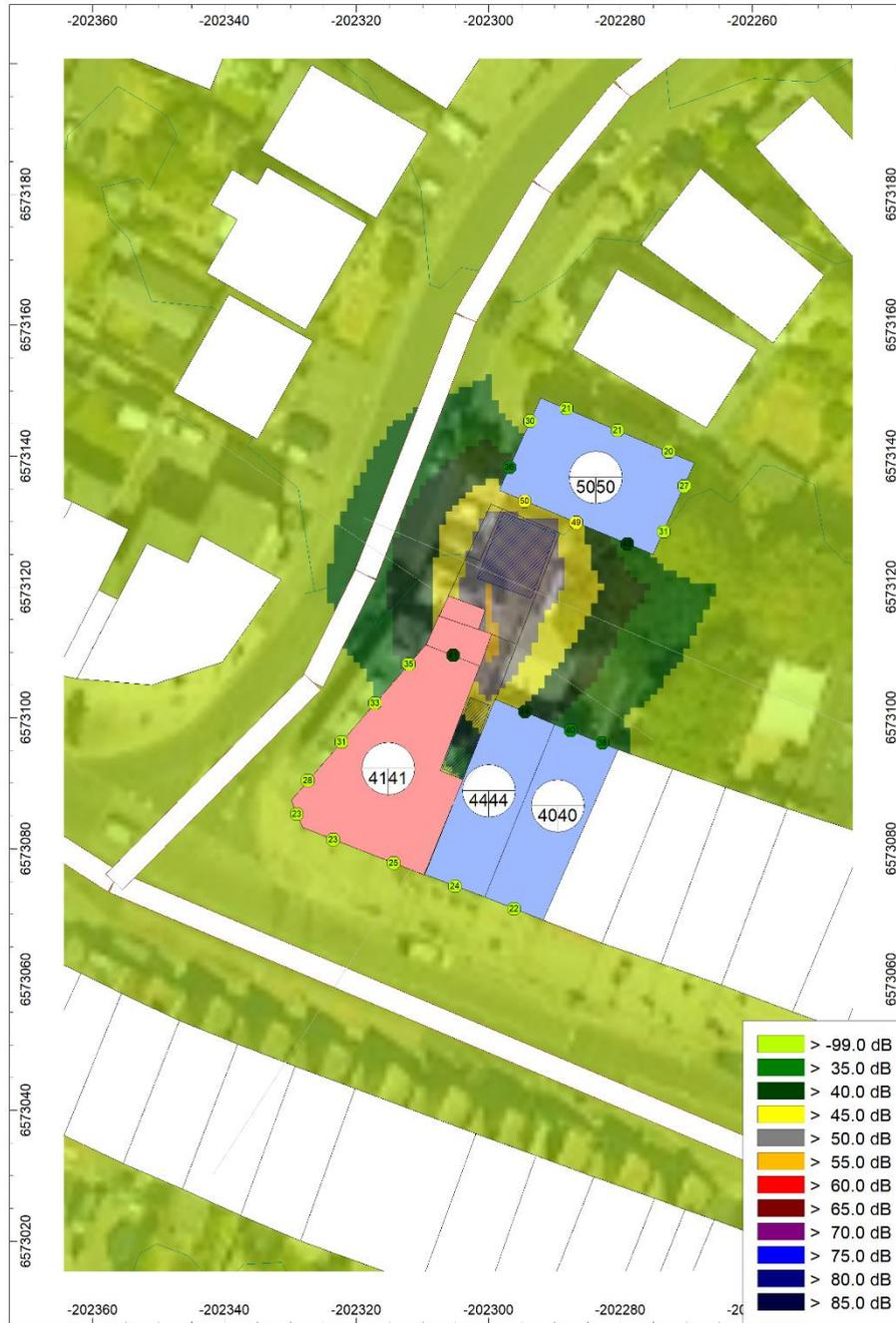
Figure 12: Plan view of beer garden model results output
